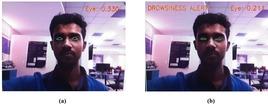
Fig 5: Figure 5(a) shows the normal state of the individual with Eye ratio above threshold ratio. In figure 5(b), Drowsiness alert message with Eye ratio below the threshold ratio has been shown.
