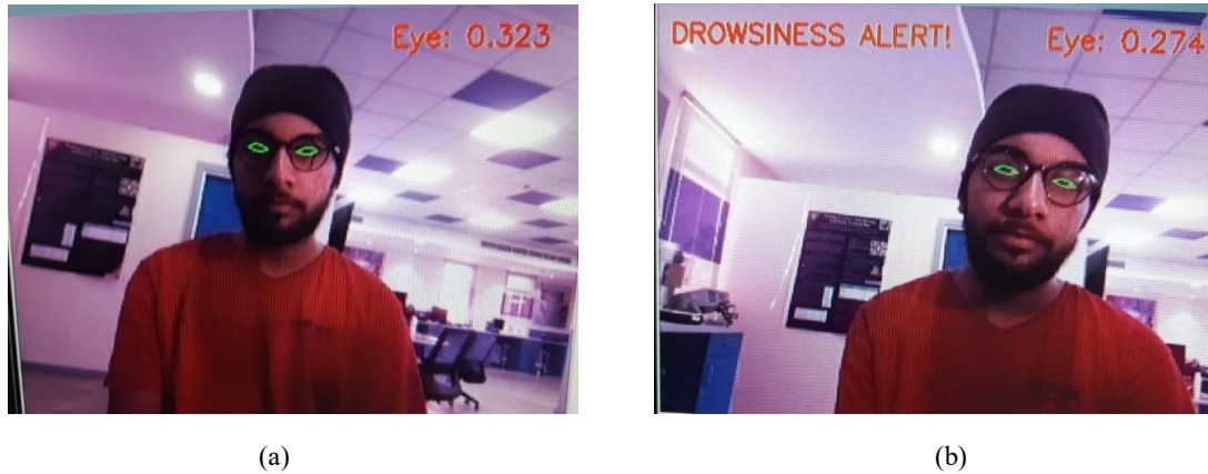
Fig.6: Figure 6(a) shows the normal state of the individual (With Spectacles) with Eye ratio above threshold ratio. In figure 6(b), Drowsiness alert message with Eye ratio below the threshold ratio has been shown.
